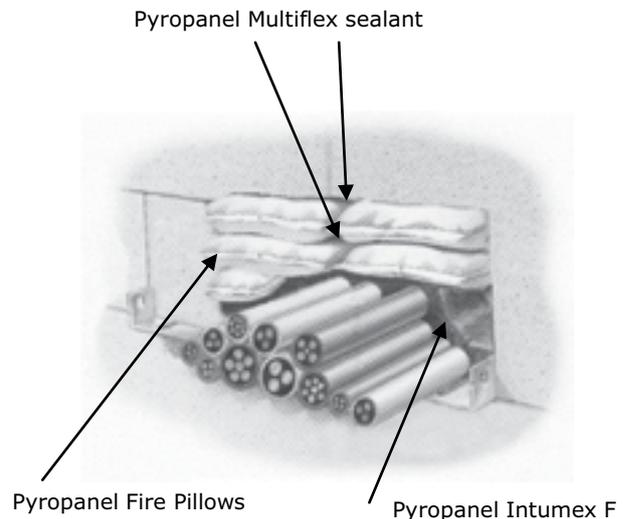
Example of P4 fire pillows sealing electrical cables and copper or ferrous pipes, in a wall penetration with Pyropanel Multiflex fire rated acrylic sealant and Pyropanel Intumex F
